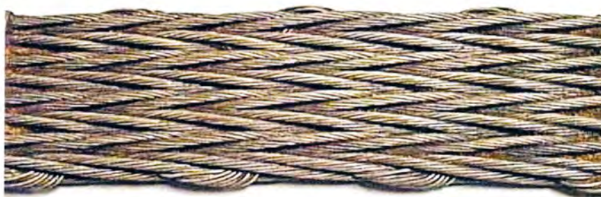
Plate 17 Flat rope, made of hemp or wire, was used for many years in winding applications. Although superseded by round wire rope it's use persisted well into the 20 th century, especially on older engines where re-fitting to accommodate round wire rope was not practical.
